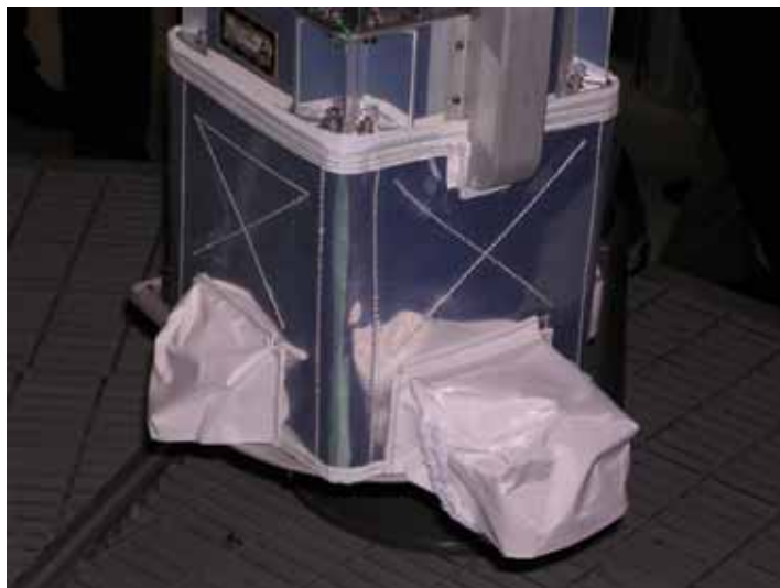
Flight Unit of Antenna Group Interface Tube (AGIT) Heat Shield. Photo by Justin Kratts
