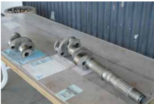
Broken crankshaft from the Stinson’s Lycoming O-435 engine. Photos by Bob Canup
