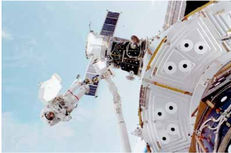
Astronaut Jim Voss installing the ECOMM antenna during the STS-102 mission. NASA photo.
