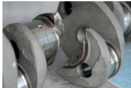
Broken crankshaft from the Stinson’s Lycoming O-435 engine. Photos by Bob Canup
