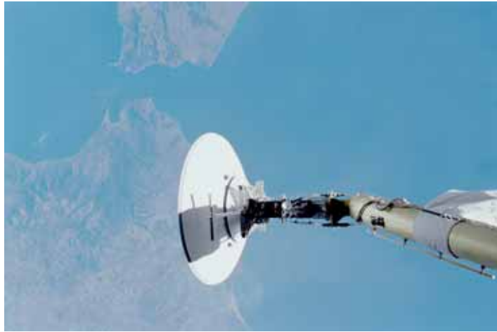
ISS Space-to-Ground Antenna (SGANT), the Station's Ku-Band antenna
