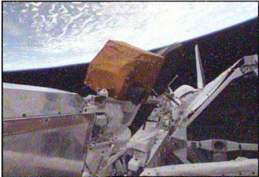
Atlantis' Ku-Band Antenna, as seen on video downlink during first orbit at ESTL
